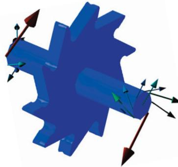
Detail Of The Total Constraint Forces On The Axle Of The Cogwheel
