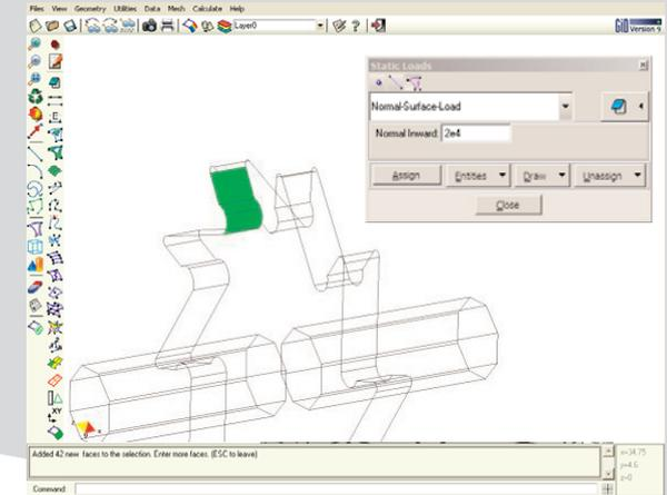
Assigning Static Loads To A Geometry Selection
